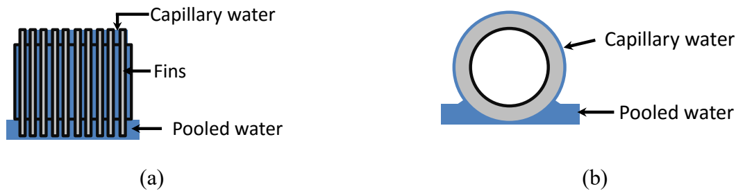
Figure 1. Capillary-assisted evaporation: (a) side view, and (b) cross-sectional view.
